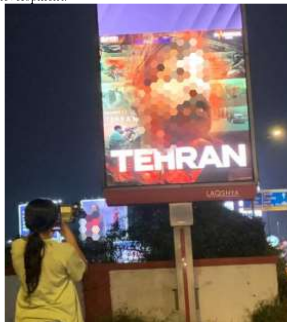
Figure 5: On-Grounds assessment of digital billboard brightness using a lux meter.
